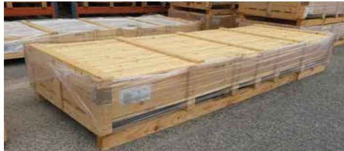
View of 3250x1170x380 mm horizontal crate with lid and runner.
