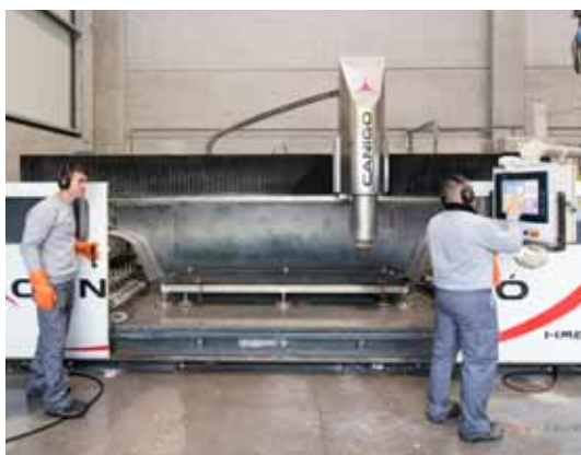
Corte y pulido del fregadero Sink cutting and polishing
